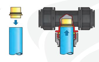
The Water Trap Tee Converter is a simple, convenient way of converting a standard 28mm Tee to a Water Trap Tee. This will stop condensing water from entering the vertical take off spur. The air supply needs to be installed with the correct fall and water drain points regularly vented.
