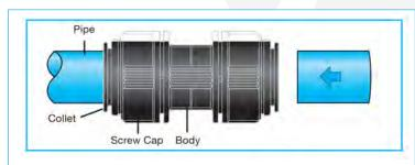
28mm fittings also have a collet with stainless steel teeth and an O-Ring.
