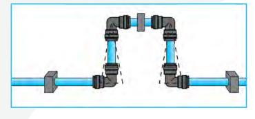
On long pipe runs, it is advisable to install an expansion bend, as shown in the diagram.
