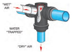
Our new Water Trap Tee solves the on-going problem of moisture in a compressed air system and provides the easy alternative to the need to install "Goose Necks". The ingenious inside arrangement of the fitting allows air to flow, with minimum head loss from the main to take-off point without allowing water to follow. The moisture is retained in the line to be drawn off at some suitable location.
